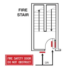
FIRE DOOR FITTED WITH A HOLD-OPEN **DEVICE: HELD IN OPEN POSITION** AND AUTOMATICALLY RELEASED BY FIRE ALARM
